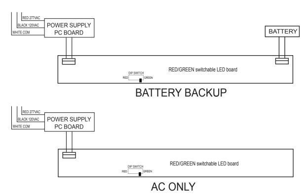
**NOTE:** Properly insulate the unused lead with a wire nut or other approved means.
