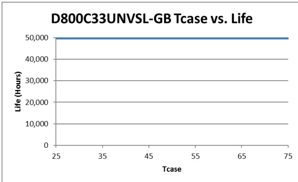
The Data curve provided predicts the LED Driver life based on the case temperature measured at the Tc location identified on the label or specification sheet. The Telecordia SR-332 standard is used to generate the prediction curves.
